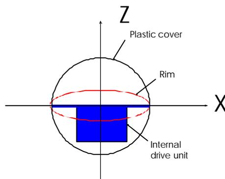
Figure 3. Functional principle of Rollo
