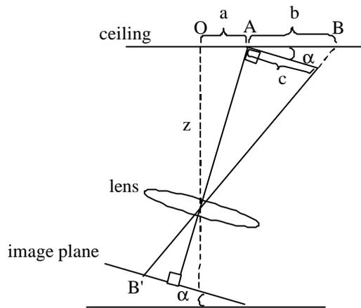
Figure 4. Using a simple camera model when image plane is tilted (one-dimensional case). **a:** Distance of the ball's position O and the point A where the normal from the lens of the camera meets the ceiling. **b:** Distance A to the known marker B on the ceiling. **c:** Normal projection of the distance b. **a:** Inclination angle in one-dimensional case.
