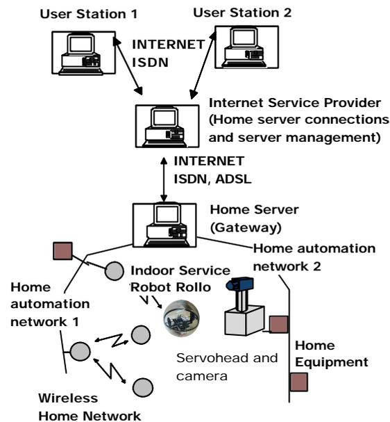
Figure 10. The Home Helper system layout consists of Internet service providers' external Internet servers, home gateways, local networks, wired and wireless local devices and home robots.
