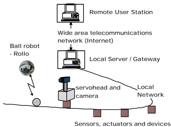
Figure 1. The Moving Eye general system structure
