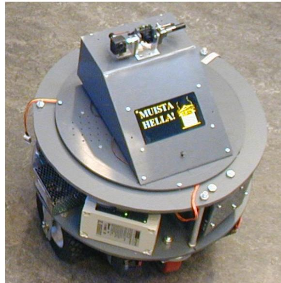
Fig. 3. Rolloottori has the same functionality as Rollo, but uses wheels for moving. It also has a touch screen which can be used as an input device.
