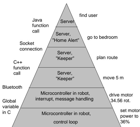
Fig. 6. Control hierarchy for moving robot in stove-alarm case
