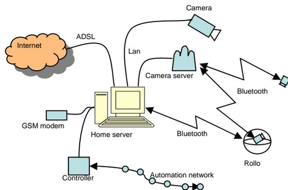
Fig. 1. General system structure
